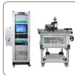
IMMERSION LAB TESTING UT
